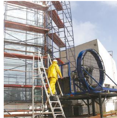
Curtain walls Test Chamber
